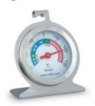
This stainless steel, fridge or freezer thermometer has a Ø50mm dial with clearly marked scale and temperature zones, indicating temperature over a range of -30 to 30°C in 1°C divisions.
